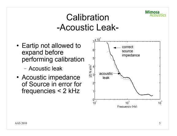
The foam eartip must be compressed before placement in the calibration cavity aperture. The foam subsequently takes a small amount of time to expand and create an acoustic seal. The figure above illustrates what happens if the calibration procedure is commenced before allowing the foam to fully expand. The acoustic impedance calculated for the probe shows an acoustic leak, the acoustic impedance of the probe being in error for frequencies less than 2 kHz.
