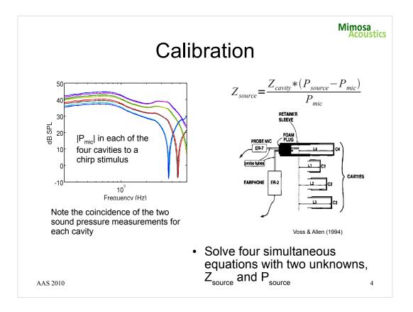
Calibration of the probe for WBR requires placing the probe in two or more cavities and measuring the sound pressure to a broad-band stimulus (in this case, a chirp). The magnitude spectrum plot shows the sound pressure measured in each of four cavities. The amplitude minima in the figure represent standing waves in the cavities. The Mimosa system uses a four-cavity calibration, as illustrated, the acoustic impedance of each cavity being known.
